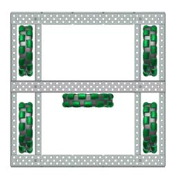
Omni-Directional wheels roll forward like normal wheels, but slide sideways with almost no friction (no skidding during turns). Use these wheels to make your robot turn smoothly or build a holonomic drivetrain.
