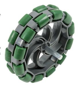
As the name suggests, an Omni-Directional Wheel can travel in more than one direction. When the axle spins, it behaves like a normal wheel. However, you'll notice that there are rollers all around the outer circumference. These rollers allow the wheel to travel sideways as well!
