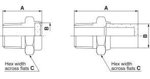
Operating temperature: –160 to 100  $^{\circ}\text{C}$
