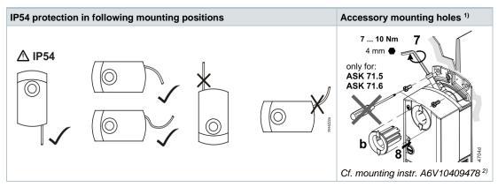
**A** 1) Not to be used for fixation of the actuator, use anti-rotation-bracket instead.
