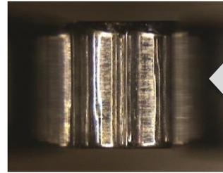
**Chromium plated crimper surface after 100,000 terminations. Note there is no visible buildup of material.**
