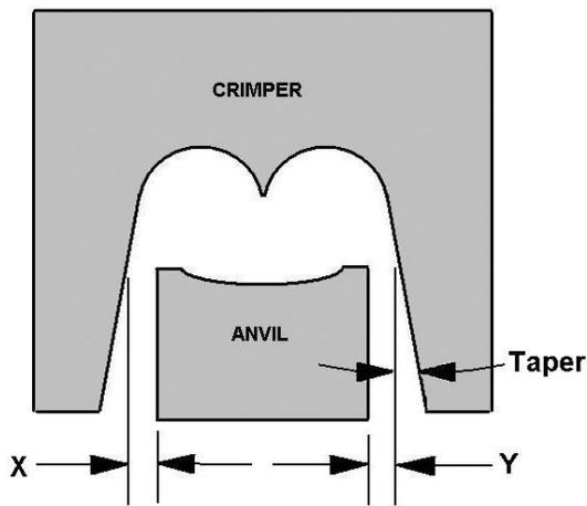
Crimper to anvil clearance is thus a combination of crimp width, crimper leg taper, anvil width, and crimp height. The critical design point is at the largest crimp height. This contribution to the gap is directly dependent on dimensional control.
