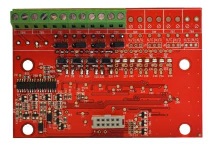
Eaton's BiWire Ultra option board is an additional daughter card that provides outputs to Fire Protection Equipment (FPE), Fire Alarm Routing Equipment (FRE) and Relays.
