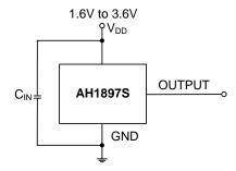
Note: 4. C<sub>IN</sub> is for power stabilization and to strengthen the noise immunity, the recommended capacitance is 100nF typical.
