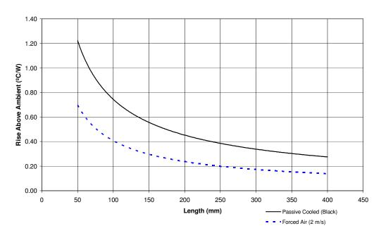
Thermal Resistance is calculated based on a distributed heat load and vertically mounted fins anodised heatsink with a 60°C temperature. Under general operating conditions the thermal mounting arrangement of devices is not known and therefore the figures should be used only as a guide to selection.
