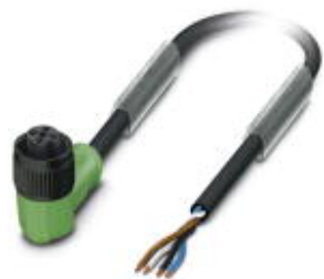
Sensor/Actuator cable, 4-position, PUR halogen-free, black-gray RAL 7021, free cable end, on Socket angled M12, A-coded, Cable length: 3 m, with plastic knurl
