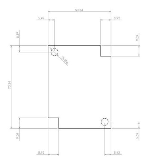
Dashed line shows outline of the mounting boss under PCB board Recommended mounting holes diameter ø3,5mm
