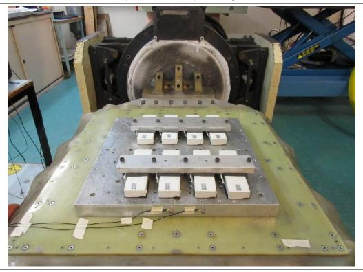
38.3.4.3: Vibration test condition-1 (Y axis direction), fixed by screws
