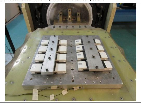
38.3.4.3: Vibration test condition-1 (Z axis direction), fixed by screws
