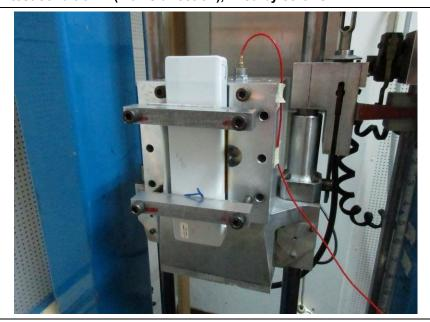
38.3.4.4: Shock test condition-2 (Y axis direction), fixed by screws
