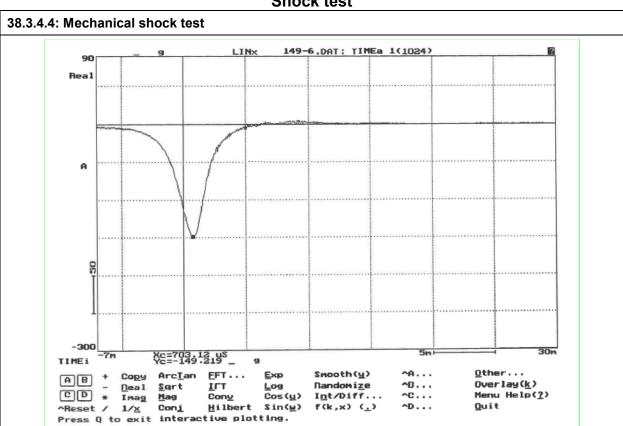
38.3.4.4: Shock test condition-1 (X axis direction), fixed by screws
