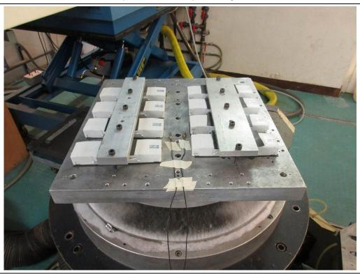
38.3.4.3: Vibration test chart-X axis direction
