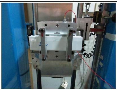
38.3.4.4: Shock test condition-3 (Z axis direction), fixed by screws
