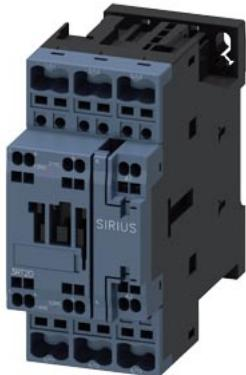
power contactor, AC-3e/AC-3, 25 A, 11 kW / 400 V, 3-pole, 230 V AC, 50/60 Hz, with plugged-in RC element, auxiliary contacts: 1 NO + 1 NC, spring-loaded terminal, size: S0
