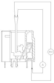
System resistance equals millivolt drop (mV) divided by test current (A) (Conductor resistance will be deducted from measurement).
