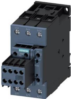
power contactor, AC-3e/AC-3, 65 A, 30 kW / 400 V, 3-pole, 175-280 V AC/DC, 50/60 Hz, with integrated varistor, auxiliary contacts: 2 NO + 2 NC, screw terminal, size: S2, removable auxiliary switch
