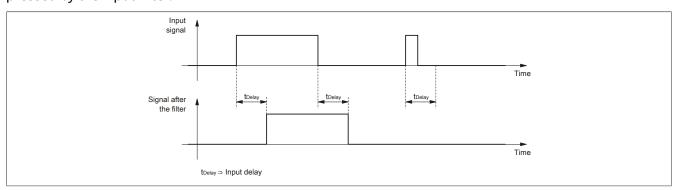
The input delay can be set in steps of 100  $\mu$ s. It makes sense, however, to enter values in steps of 2 since the input signals are sampled in an interval of 200  $\mu$ s.
