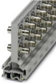
BNC connector, double-level, for mounting on NS 32 or NS 35/7.5, wave impedance: 50 Ohm
