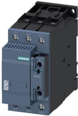
capacitor contactor, AC-6b 75 kVAr, / 400 V, 3-pole, 175-280 V AC/DC, 50/60 Hz, with integrated varistor, auxiliary contacts: 2 NC, screw terminal, size: S2
