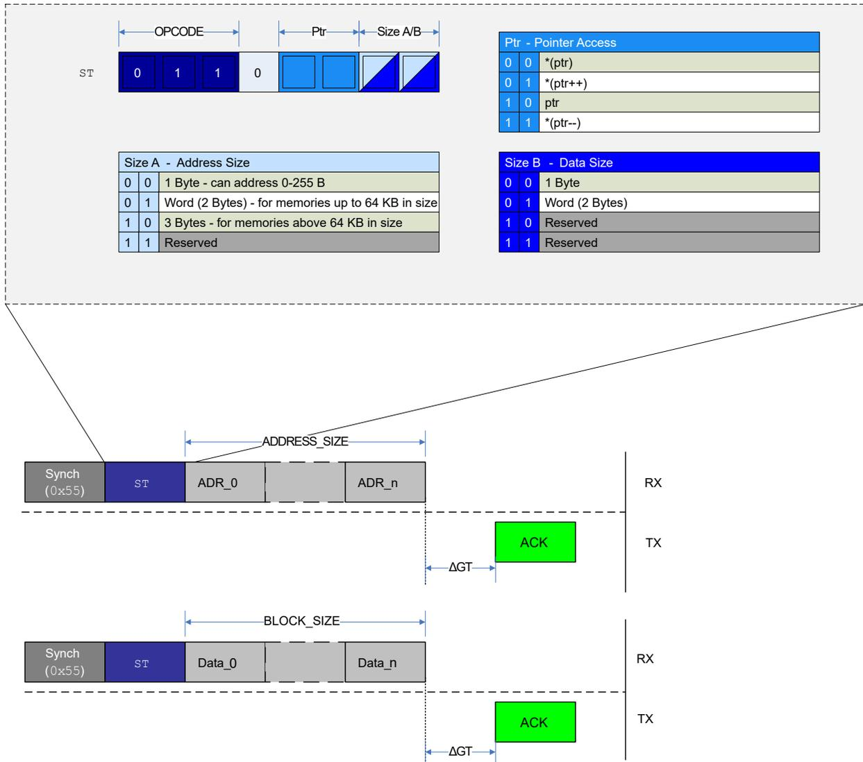
Figure 33-12 gives an example of an `ST` instruction to the UPDI Pointer register and the storage of regular data. A SYNCH character is sent before each instruction. In both cases, an Acknowledge (ACK) is sent back by the UPDI if the `ST` instruction was successful.
