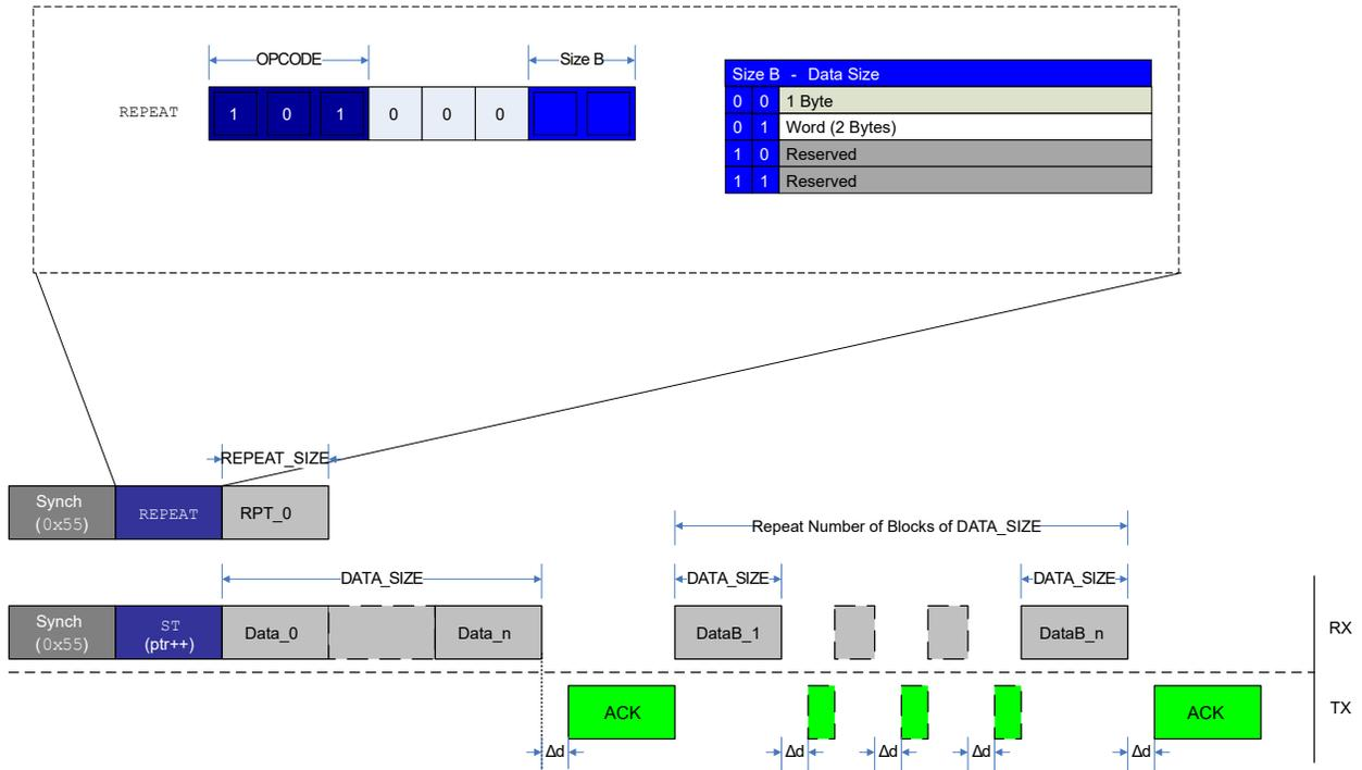
Figure 33-15 gives an example of a repeat operation with an ST instruction using pointer post-increment operation. After the REPEAT instruction is sent with RPT\_0 = n, the first ST instruction is issued with SYNCH and instruction frame. The next n ST instructions are executed by only sending data bytes according to the ST operand DATA\_SIZE and maintaining the Acknowledge (ACK) handshake protocol.
