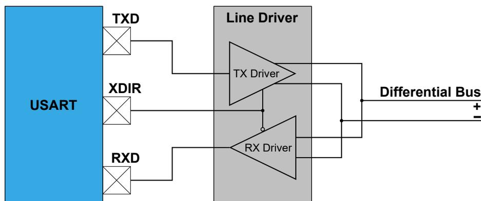
The XDIR pin goes high one baud clock cycle in advance of data being shifted out to allow some guard time to enable the external line driver. The XDIR pin will remain high for the complete frame, including Stop bit(s).
