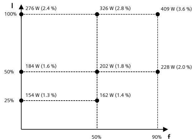
**NEC power loss data based on**
