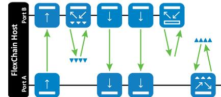
FlexChain, the individual light grid: Whether through-beam photoelectric sensors, photoelectric retro-reflective sensors or photoelectric proximity sensors – the sensor technology can be freely selected and combined.
