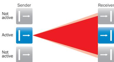
Optimum measurement certainty: Sequential cycling prevents the signals from overlapping
