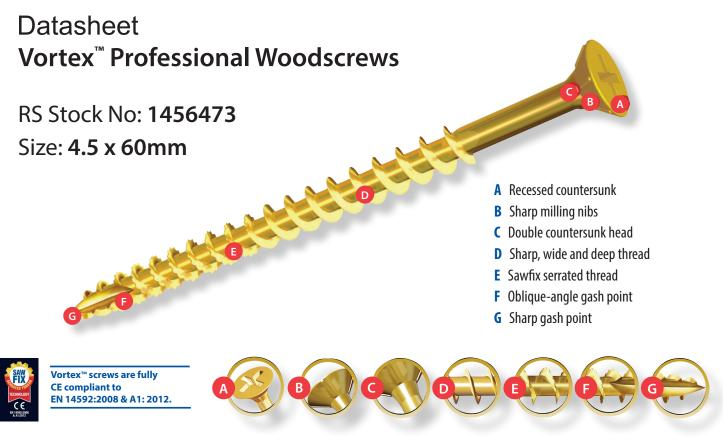
The recessed double countersunk head on the Vortex<sup>™</sup> product range reduces the likelihood of shearing the head of the screw, whilst assisting the completion of countersinking, making it a more reliable product for users.
