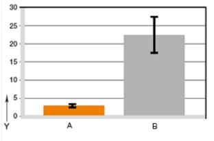
Wear rotating against stainless steel pin (1.4305) F= 35 N, v= 0,5 m/min
