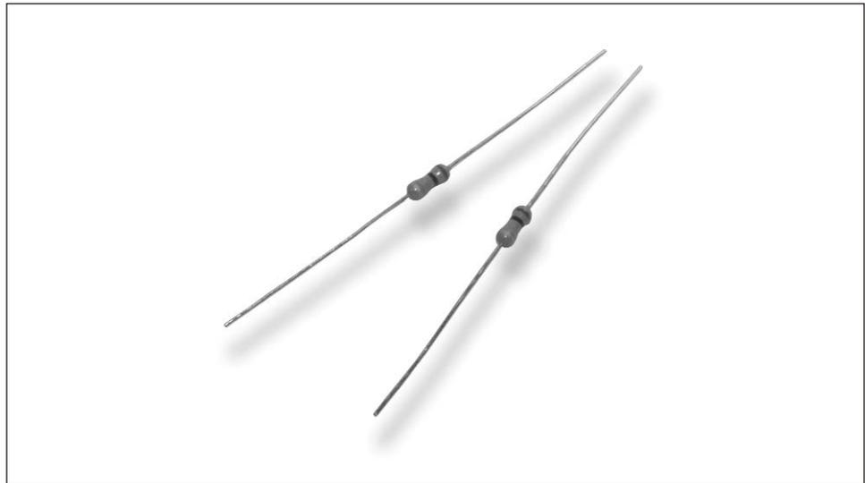
Metal glaze resistors are manufactured using thick film techniques. The ceramic slugs have the thick film applied, the film is fired and end caps are forced onto the slugs, the resistive element is spiralled to value and lead wires are welded onto the end caps. Four layers of coating are applied - the first being a phenolic resin, the other three being epoxy.
