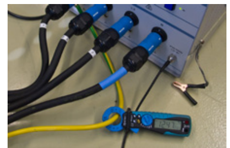
Fig. 4: Measuring current on a ground conductor (source: SCHURTER AG)
