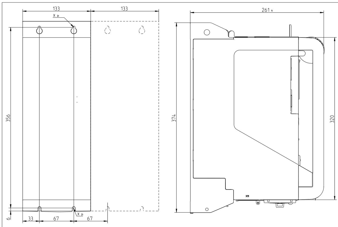
Figure 2: SafeMOTION double-width modules - Dimension diagram
