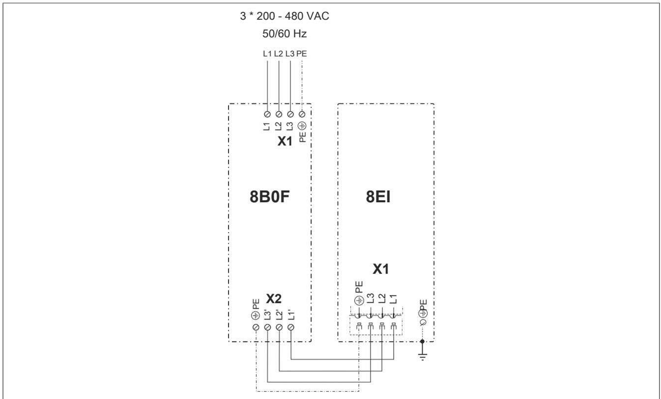
Figure 5: Mains connection 3x 200 - 480 VAC
