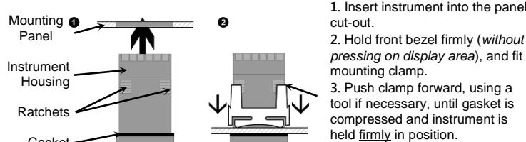
**CAUTION:** For an effective IP65 seal against dust and moisture, ensure gasket is well compressed against the panel, with the 4 tongues located in the same ratchet slot.
