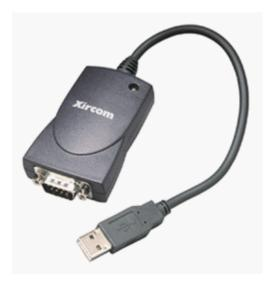
The USB to Serial Converter allows you to use all Pico Technology serial dev such as TC-08, ADC-16, EnviroMon and other serial devices through the USI on your PC. Installation is simple. Plug your serial device into the Converter. converter into your computer. Insert the disk. With USB technology, there ar IRQ conflicts and no COM Port conflicts.
