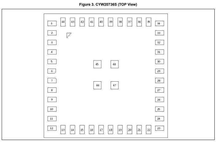
The signal name, type, and description of each pin in the CYW20736S is listed in Table 3 on page 6. The symbols shown under I/O Type indicate pin directions (I/O = bidirectional, I = input, O = output) and the internal pull-up/pull-down characteristics (PU = weak internal pull-up resistor and PD = weak internal pull-down resistor), if any.
