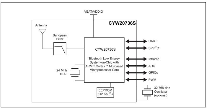
Figure 1. CYW20736S BLE SiP Block Diagram
