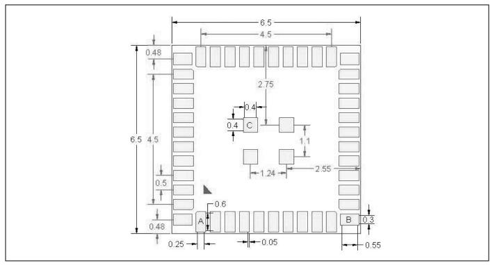
Figure 15. CYW20736S Pin Dimensions (Bottom View)
