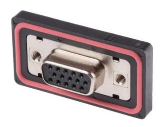
The RS PRO series of waterproof D-sub connectors are a range of ruggedised IP67 connectors designed to be used outdoors or in harsher industrial environments. Designed to fit panel cut outs of 40.0mm the waterproof D-sub series also comes with rear potting on the panel mount connectors. This ensures your panel is still sealed to an IP67 rating even when the connector is unmated. The Push-Fit with dual Screws mating allows for a secure connection.
