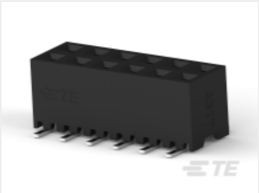
TE Part # 1-2307819-4 14P,2MM,BB,REC,DRV,SM,0.76AU, TR,W/CP
