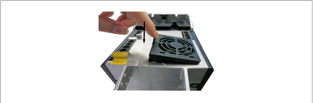
Figure 92: Installing the fan module
