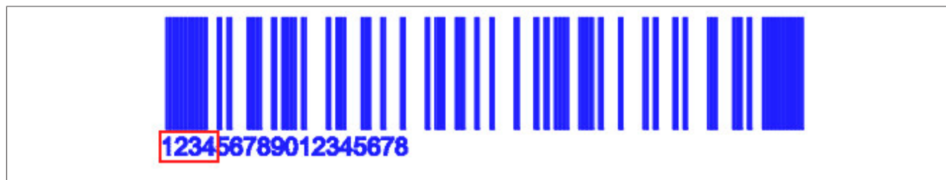
Figure 2: B&R ID code (marked) as part of the serial number
