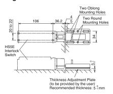
Fasten the actuator cover on at least two rectangular holes and two round mounting holes using mounting screws. The thickness adjustment plate requires mounting holes.
