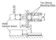
Fasten the actuator cover on at least two oblong holes using mounting screws.
