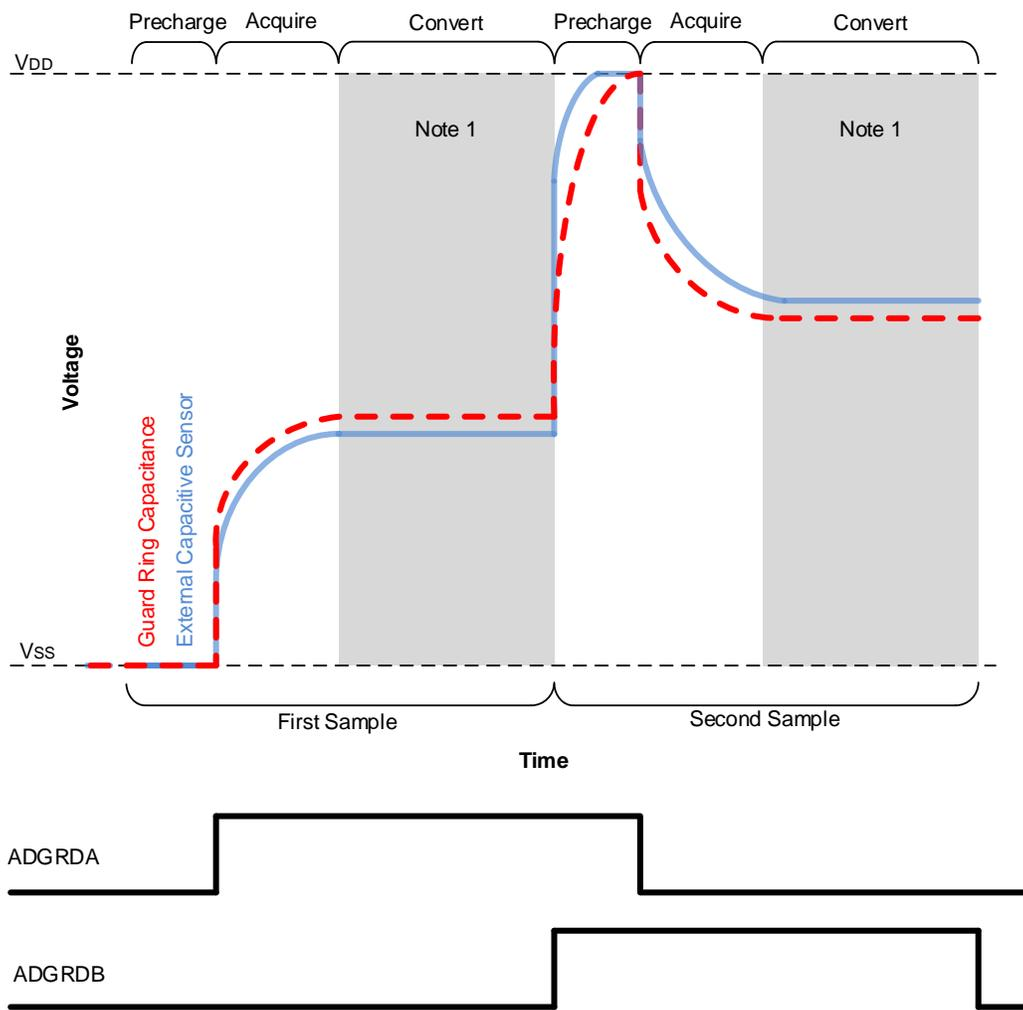
Note 1: External Capacitive Sensor voltage during the conversion phase may vary as per the configuration of the corresponding pin.
