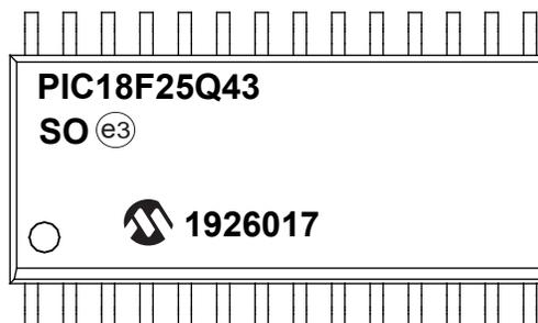
28-Lead SSOP (5.30 mm)
