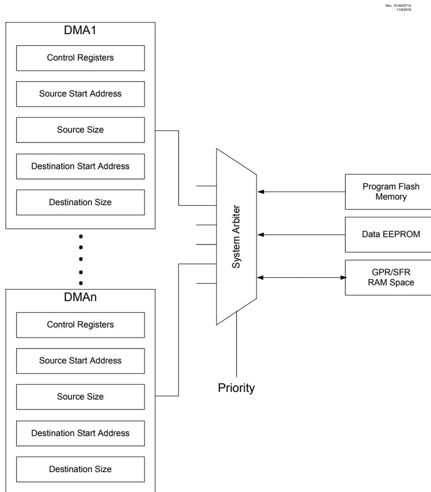
Depending on the priority of the DMA with respect to CPU execution (refer to the **“Memory Access Scheme”** section in the **“PIC18 CPU”** chapter for more information), the DMA Controller can move data through two methods:
