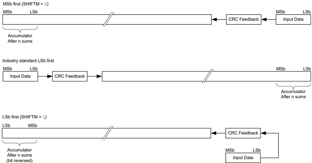
When **SHIFTM** is not set, the data will be shifted in MSb first and the result will be big-endian. When **SHIFTM** bit is set, the data will be shifted into the accumulator in reversed order, LSb first and the result will be little-endian.
