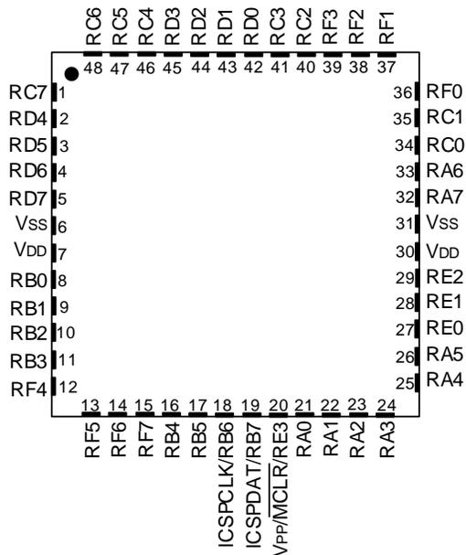
**Note:** It is recommended that the exposed bottom pad be connected to V<sub>SS</sub>; however, it must not be the only V<sub>SS</sub> connection to the device.
