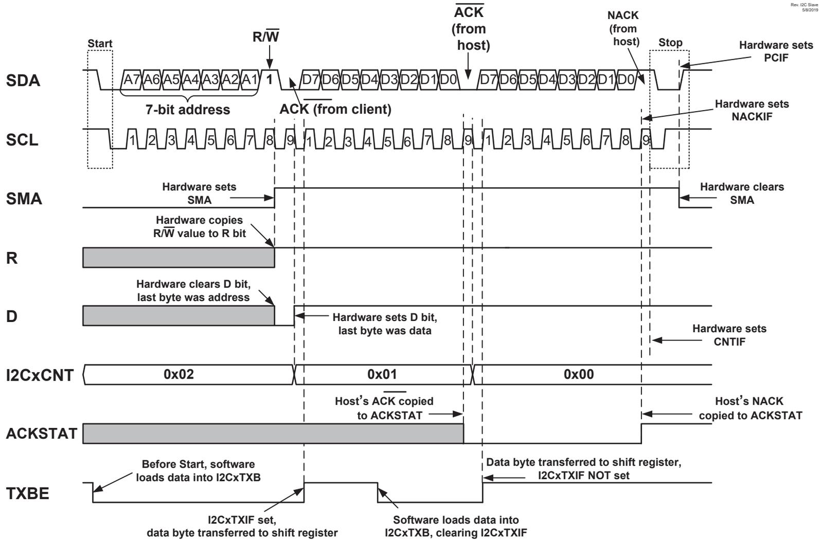
Figure 36-14. 7-Bit Client mode Transmission (ADRIE = 1)
