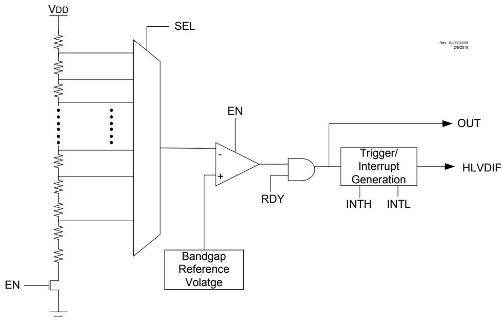
Since the HLVD can be software enabled through the [EN](#) bit, setting and clearing the enable bit does not produce a false HLVD event glitch. Each time the HLVD module is enabled, the [RDY](#) bit can be used to detect when the module is stable and ready to use.
