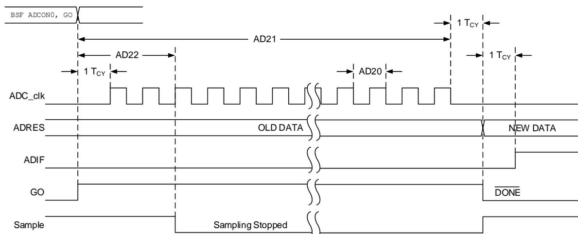
Figure 47-10. ADC Conversion Timing (ADC Clock from ADCRC)
