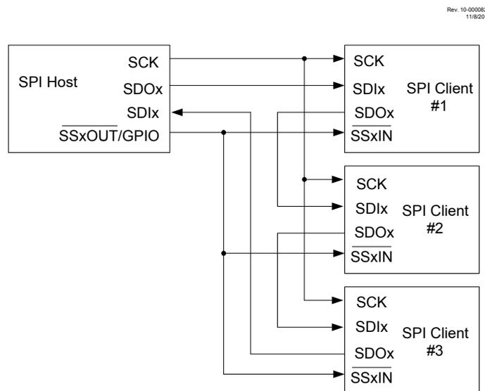
**Figure 35-13.** SPI Daisy-Chain Connection with Chained SCK
