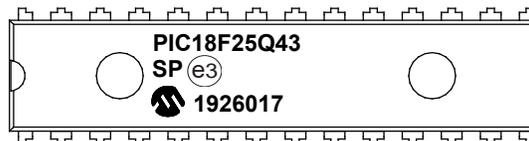
28-Lead SOIC (7.50 mm)
