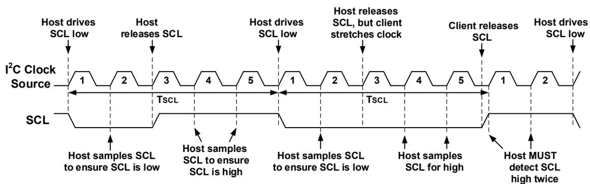
When FME is set (FME = 1), one SCL period ( $T_{SCL}$ ) is equal to four clock periods of the selected I2CxCLK source. In other words, the I2CxCLK source is divided by four. Using the example from above, if the MFINTOSC (500 kHz) clock source is selected and the FME bit is set, the actual SCL frequency is 125 kHz (see Equation below).
