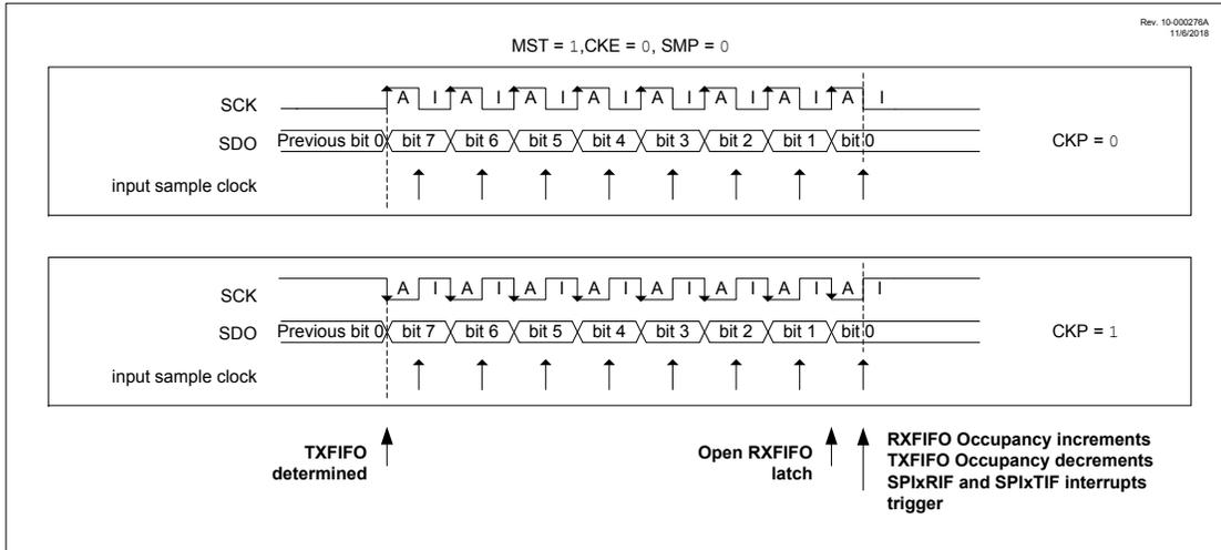
**Figure 35-8.** Clocking Detail - Host Mode, CKE = 1, SMP = 1
