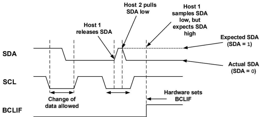
**Figure 36-42. Multi-Host Mode Transmission**
