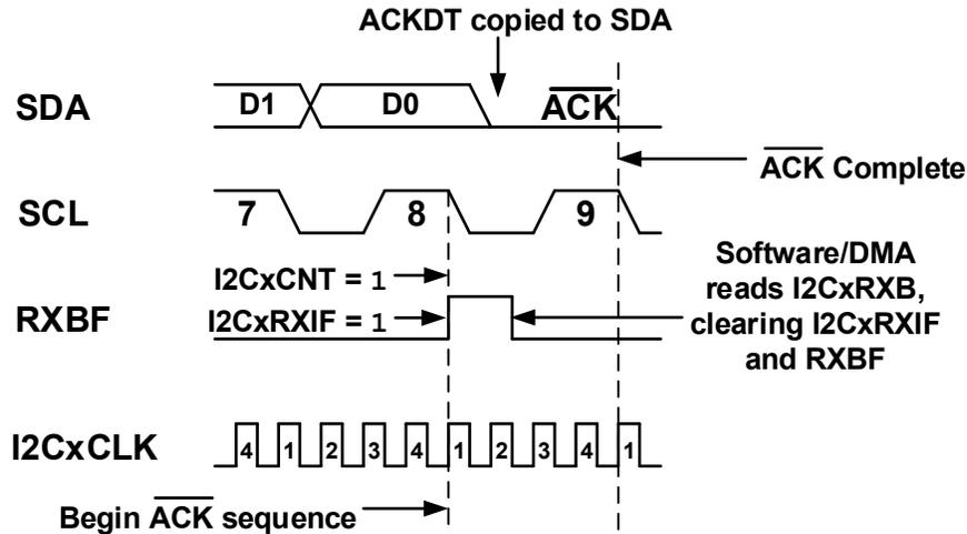
Figure 36-33. Not Acknowledge (NACK) Sequence Timing
