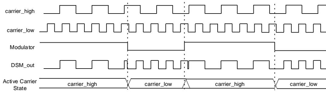
**Figure 33-6.** Full Synchronization (CHSYNC = 1, CLSYNC = 1)
