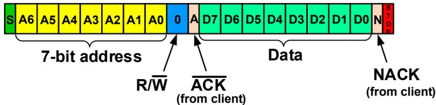
Figure 36-27. 7-Bit Host Write Diagram (To a Specific Memory/Register Location)
