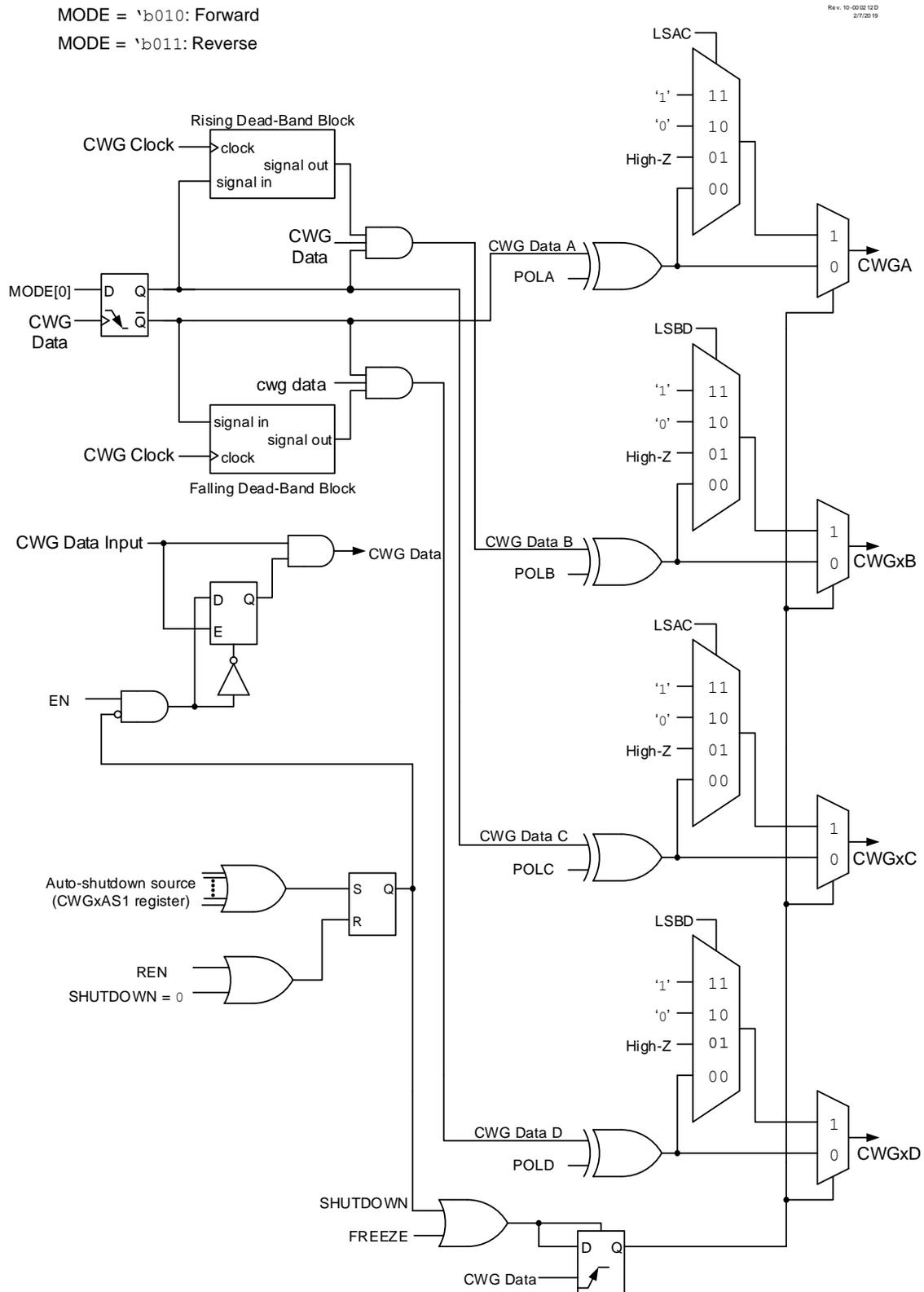
In Forward Full Bridge mode ( $MODE = \text{'b}010$ ), CWGxA is driven to its Active state, CWGxB and CWGxC are driven to their Inactive state, and CWGxD is modulated by the input signal, as shown in Figure 31-7.
