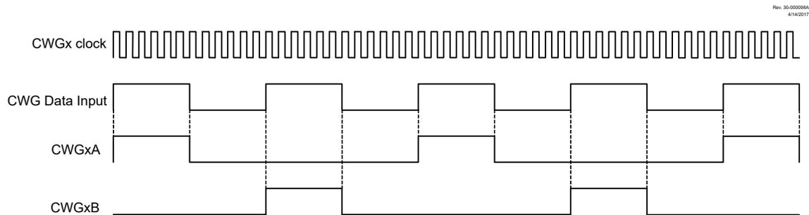
Figure 31-4. Simplified CWG Block Diagram (Push-Pull Mode, MODE = `b101)
