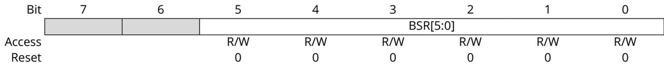
**Bits 5:0 – BSR[5:0]** Most Significant bits of the data memory address
