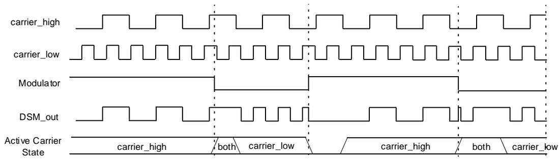
**Figure 33-5.** Carrier Low Synchronization (CHSYNC = 0, CLSYNC = 1)
