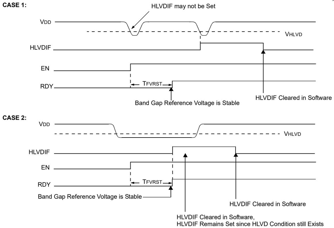
Figure 37-3. High-Voltage Detect Operation (INTH = 1)
