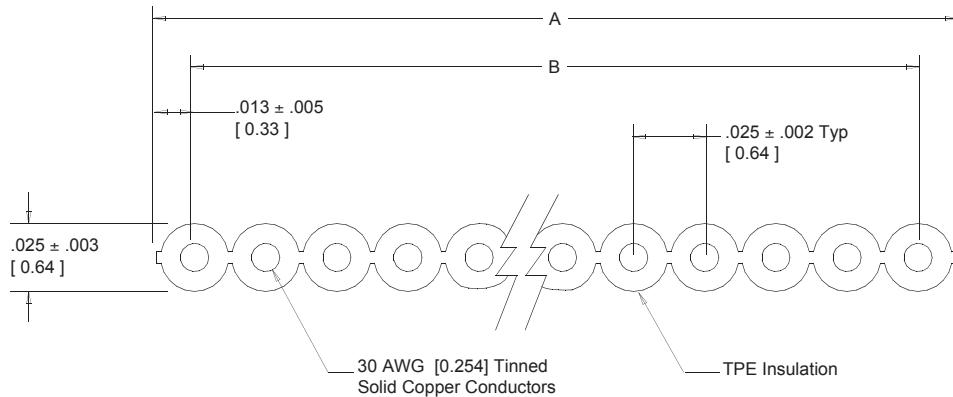
Note: Blue marking on one edge of cable designates wire #1.
