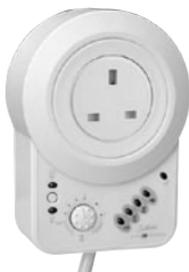
The AVS is an Automatic Voltage Switcher rated at 13 Amps (AVS13) or 15Amps (AVS15). The AVS will switch off the equipment connected to it if the mains power goes outside preset acceptable limits and will re-connect -automatically\* - when the mains power returns to normal. Re-connection takes place after a delay to ensure stability of the mains.
