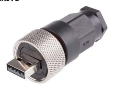
The RS PRO series of waterproof metal USB-A connectors are a range of ruggedised IP67/IP68 connectors designed to be used outdoors or in harsher industrial environments. Designed to fit panel cut outs of 25.5mm the metal USB-A series also comes with rear potting on the panel mount connectors. This ensures your panel is still sealed to an IP67/IP68 rating even when the connector is unmated, and the sealing cap is not connected. The threaded mating allows for a secure connection.
