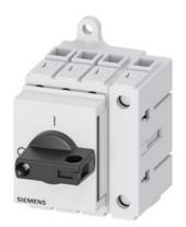
Load disconnector 3LD3, Iu 40 A Main switch 3-pole + N Rated operating capacity at AC-23 A at 400 V 18.5 kW Installation in distribution boards, Basic switch with selector knob black
