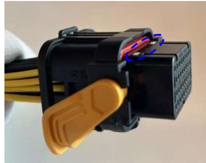
Final lock in final lock (The white protrusion is flush with the Socket insulator) 终锁在终锁位置(白色凸点与绝缘座齐平)
