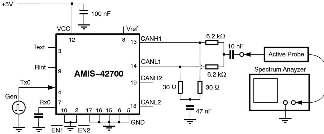
Figure 9. Basic Test Set-up for Electromagnetic Measurement
