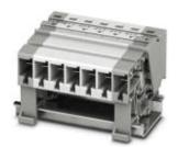
COMBI receptacle, Connection method: Push-in / plug connection, Number of positions: 1, Cross section: 0.5 mm² - 10 mm², AWG: 20 - 8, Width: 8.2 mm, Color: gray, Mounting type: NS 35/15, NS 35/7,5
