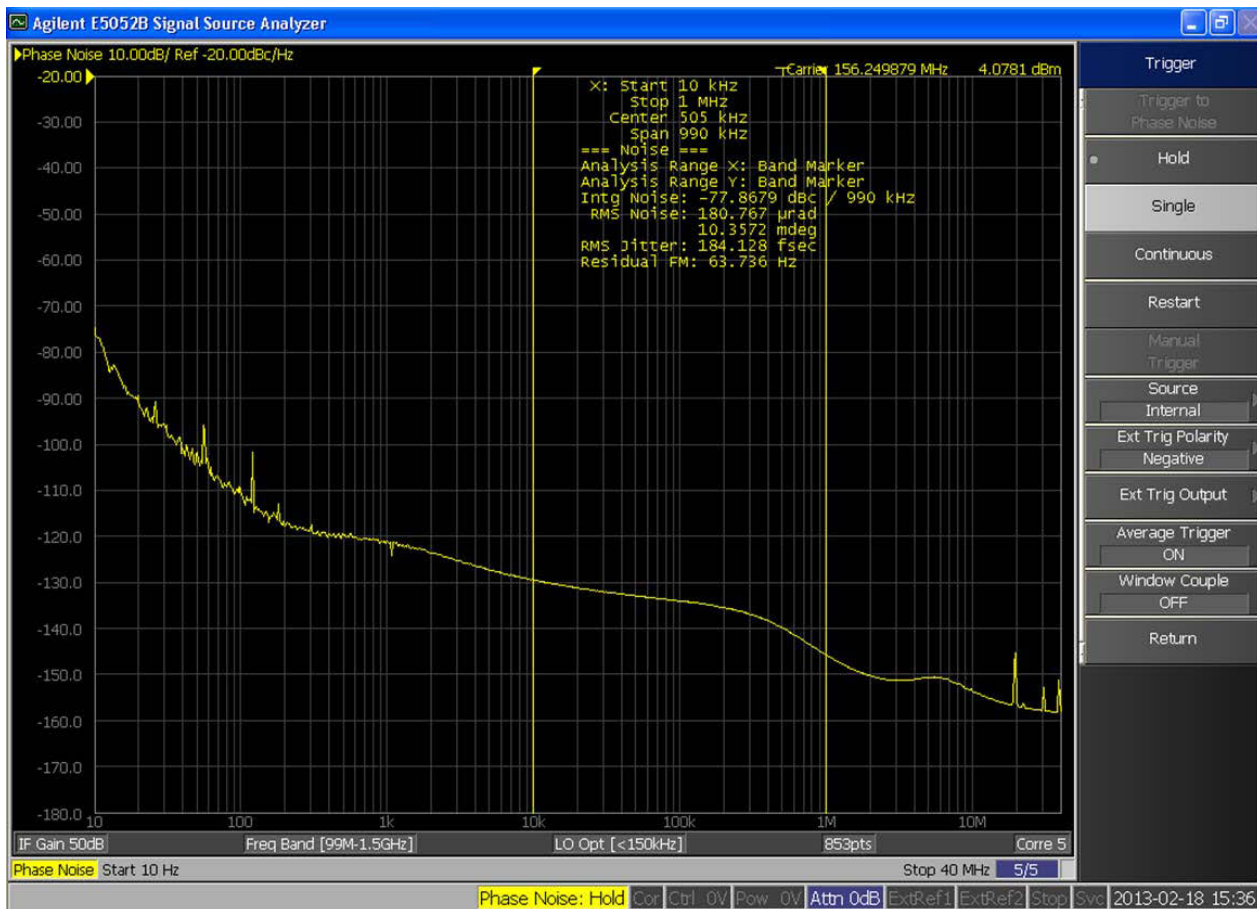
Figure 1. Si535/536 Typical Phase Noise at 156.25 MHz
