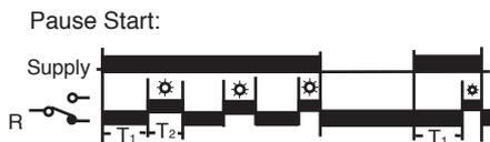
When the supply is connected and the set pause time has elapsed the output relay 'R' is energised. 'R' remains energised for the set pulse time period. The sequence repeats until the supply is interrupted.
