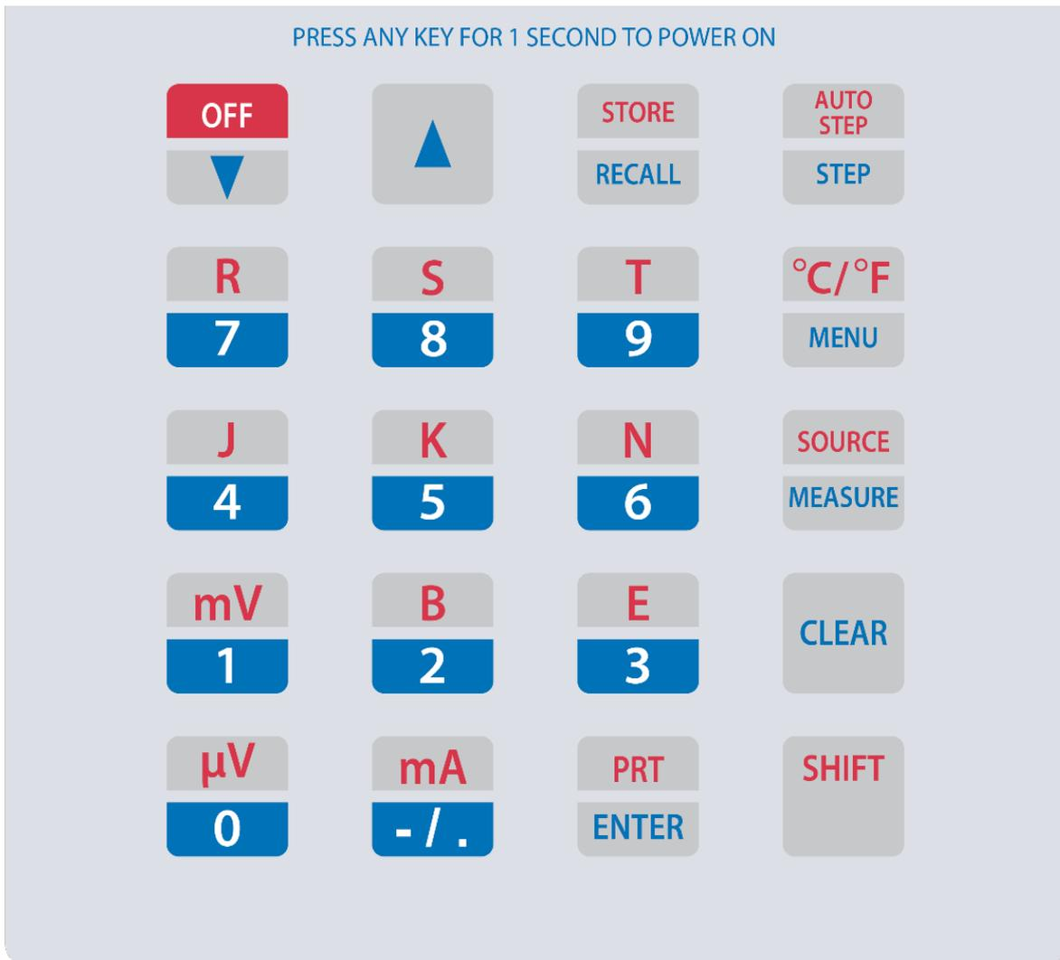
**Note:** The secondary keypad functions are available only when relevant to the selected operating mode. For example: 'Auto Step' is not available when the 1090 is in measure mode.
