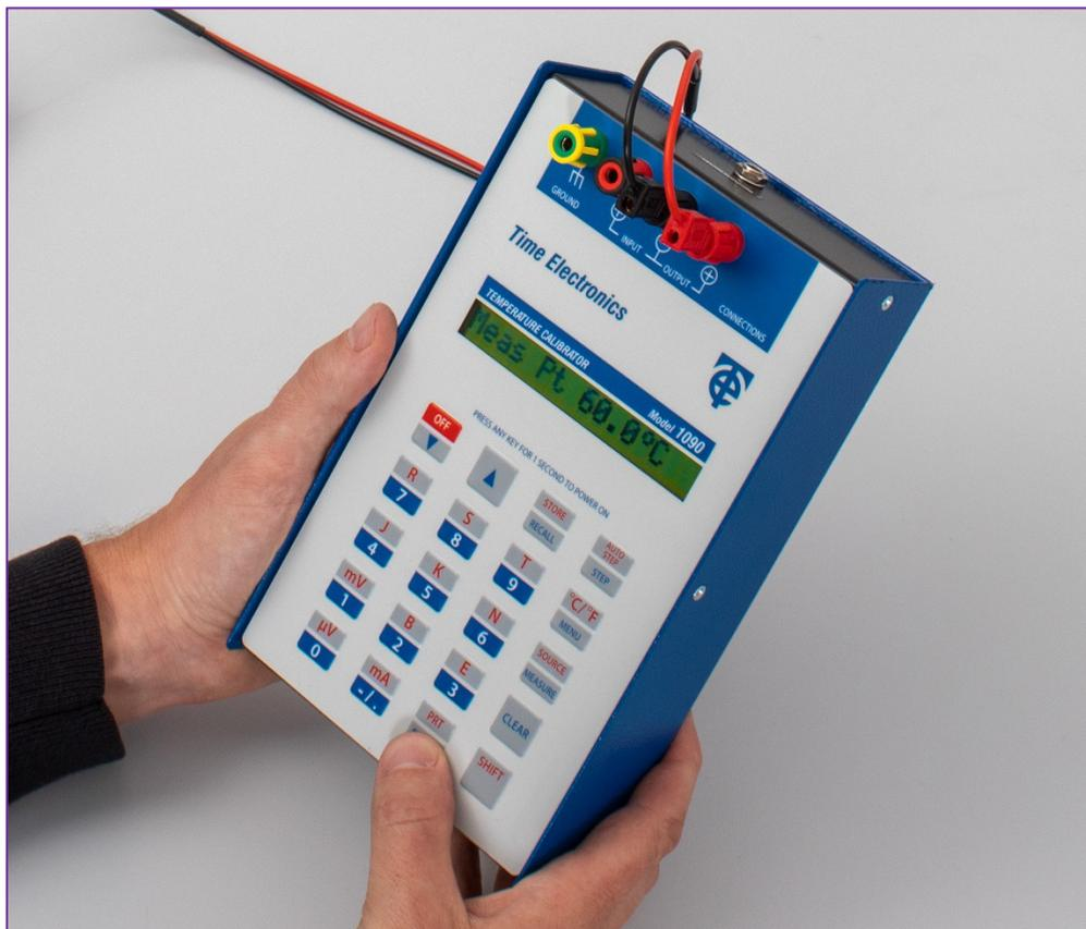
The 1090 is a high-performance instrument designed for use in both the lab and field applications. It simulates and can measure from the most commonly used temperature sensors - thermocouples (8 types) and Pt100.
