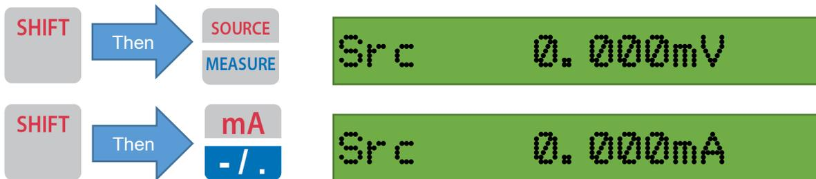
Enter the desired mA values using the numbered keys or 'Up/Down' arrow keys.
