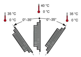
A maximum ambient temperature of +40  $^{\circ}$ C is permitted for vertical mounting (0 $^{\circ}$  tilt angle); a maximum of +35  $^{\circ}$ C is permitted for inclined mounting.
