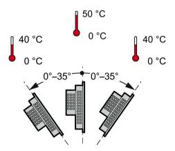
A maximum ambient temperature of +50 °C is permitted for vertical mounting (0° tilt angle); a maximum of +40 °C is permitted for inclined mounting.
