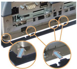
3. Insert the mounting seal into the stainless steel front as shown. Also note points ④ - ⑥.
