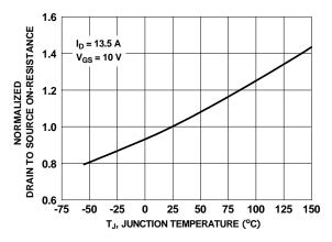
Figure 3. Normalized On-Resistance vs Junction Temperature
