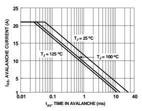
Figure 9. Unclamped Inductive Switching Capability
