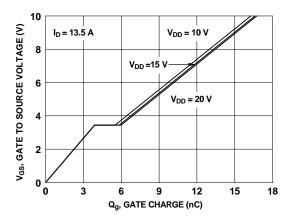
Figure 7. Gate Charge Characteristics
