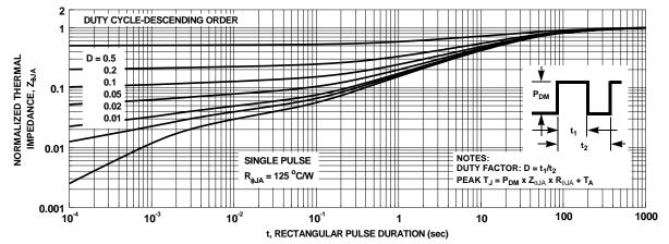
Figure 13. Junction-to-Ambient Transient Thermal Response Curve
