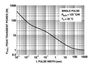
Figure 12. Single Pulse Maximum Power Dissipation
