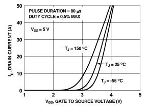
Figure 5. Transfer Characteristics
