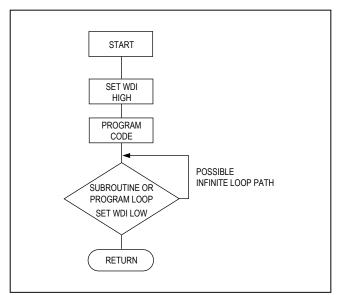
Figure 3. Watchdog Flow Diagram
