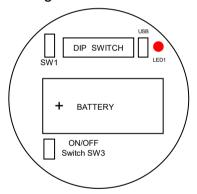
Switches 1, 2, 3 & 4 select the RF Network the IWPTL will transmit on. The default network for both the IWPT transmitter and IWR receiver is network 1.
