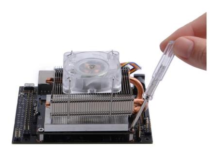
5. Connect fan to mainboard on J15 as following picture, please beware of the direction of the cable.
