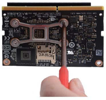
3. Fixed the Ice tower radiator to the mainboard with screws and please pay attention to the direction of mounting racket.
