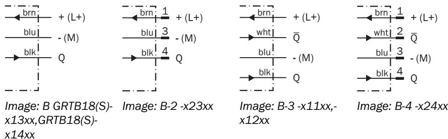
Only apply voltage / switch on the power supply ( $V_S > 0$  V) once all electrical connections have been completed. The green LED indicator lights up on the sensor. Explanations of the connection diagram (graphic B):
