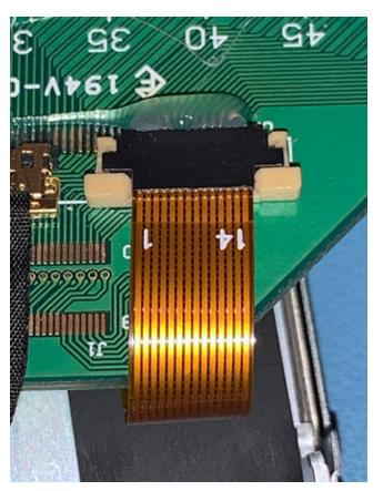
The connections should look like this when the connectors are connected correctly
