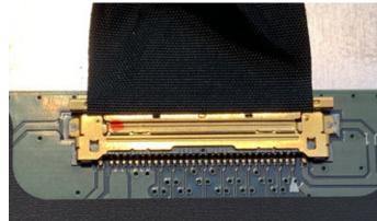
The connection should look like this when the connector is connected correctly.
