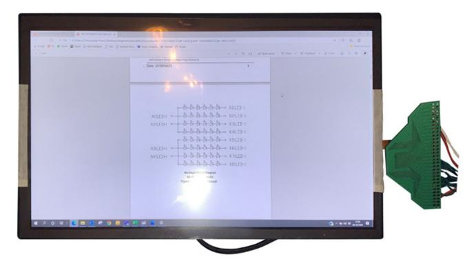
The connections are very fragile and easily torn. It is recommended that all connections are taped and all loose parts are insulated and taped to the rear of the display once the connections have been completed.
