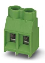
PC terminal block, Nominal current: 32 A, Nom. voltage: 500 V, Pitch: 7.62 mm, Number of positions: 2, Type of connection: Screw connection, Assembly: Soldering, Conductor/PCB connection
